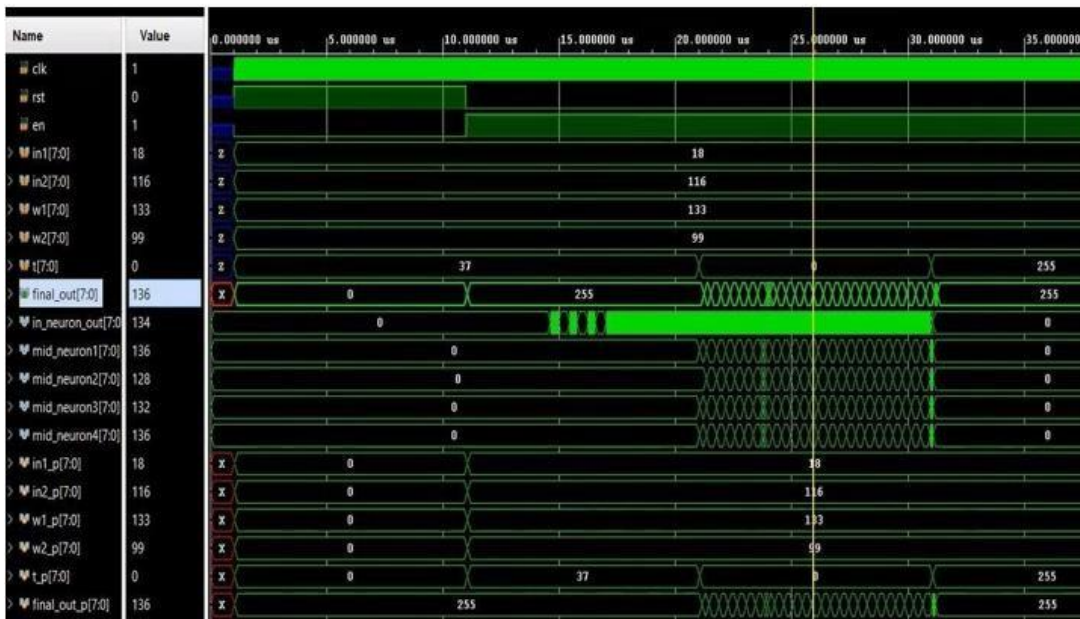
Figure.7. Simulation result of single neuron column model
